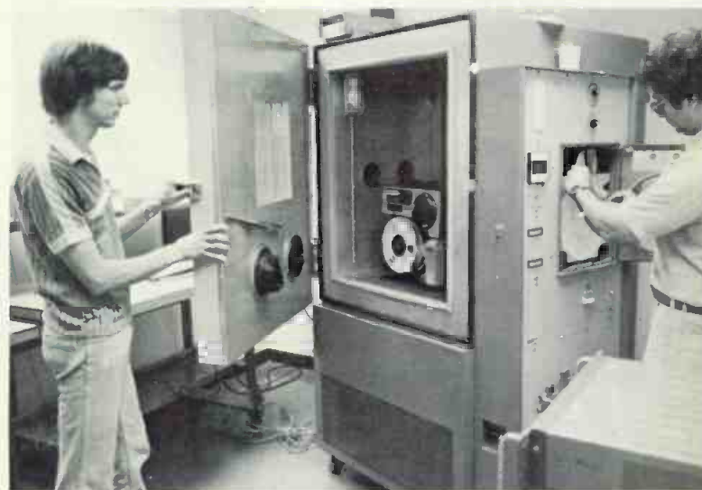
The recorder is environmentally tested in anticipation of future operating demands
