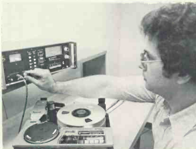
ABC employs an Asaca/ShibaSoku color video noise meter to measure signal-to-noise ratio
